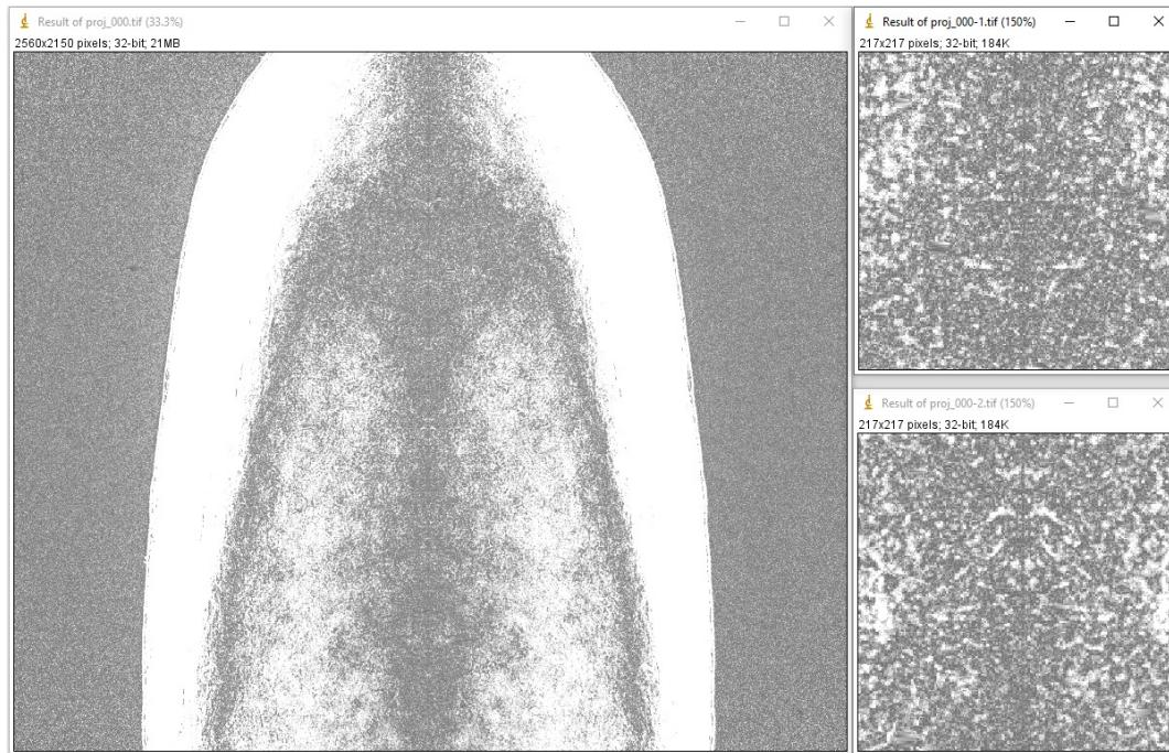
If a tilt is detected, the tilt angle can be accurately calculated by locating the center of rotation using sinograms generated at the top, middle, and bottom of the FOV; then applying a linear fit to the results. The resulting tilt angle can be used to correct the tilted tomographic images, as shown [here](#).
